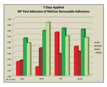
The chart above compares 90 degree peel-adhesion of current Mactac removable adhesives, 1001 and HR51, to our newest Mactac Removable adhesives, MR840 and MR860, applied and removed after seven days. Knowing your end-use application will help in selecting the Mactac Removable that is right for you.
