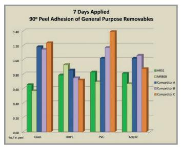
The chart above compares Mactac's two general purpose removables, HR51 and MR860, to three competitor products. With removable adhesive the lower the peel value, the simpler it is to remove the label. With this in mind, it's easy to see that Mactac general purpose removables consistently outmatch the competition.
